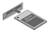
\* The type of flash memory card required for use in the LCD projector is a Type II PCMCIA-ATA flash memory card (not supplied). Never use other types of PC card than this. Doing so can break the slot or ruin the PC card.
